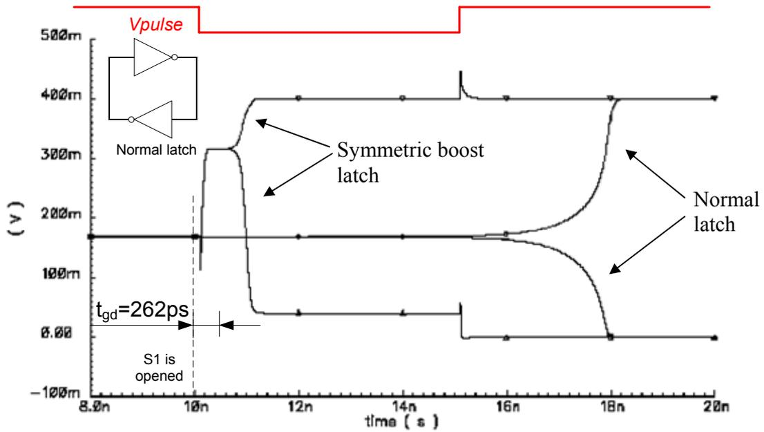
Figure 22 Transient analysis,  $V_{DD}=0.4V$ ,  $T=-20^{\circ}C$
