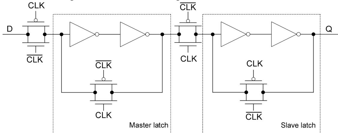
**Figure 1 Typical Edge Triggered D Flip-Flop**
