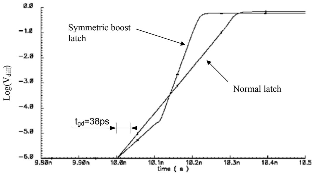
Figure 21  $\tau$  calculation,  $V_{DD}=0.7\text{V}$ ,  $T=-20^\circ\text{C}$ .  $\tau$  (symmetric boost)=11ps,  $\tau$  (Normal latch)=24ps.
