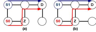
Figure 7. XYDT Examples: (a) No routing table entries (b) One routing table entry in node Z towards destination D
