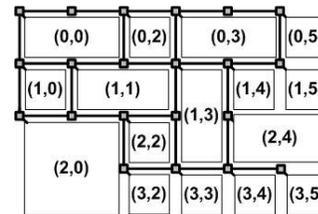
Figure 1. SoC interconnected by irregular mesh NoC. The address of each module corresponds to its top left corner coordinates.
