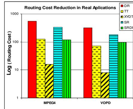
Figure 10. The routing costs on real video processing application examples: up to 40X cost reduction by XYDT; and 2.9X by SRDP
