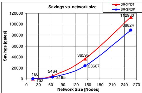
Figure 11. Savings vs. network size in typical NoC
