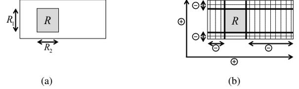
Fig. 5. Two-dimensional range  $R = (R_1, R_2)$ . Fig. 5(a) presents the encoding of the two-dimensional range  $R$  using an internal encoding, yielding an expansion which is exponential in the number of fields. Fig. 5(b) demonstrates the encoding of  $R$  using the suggested encoding which yields a linear expansion.
