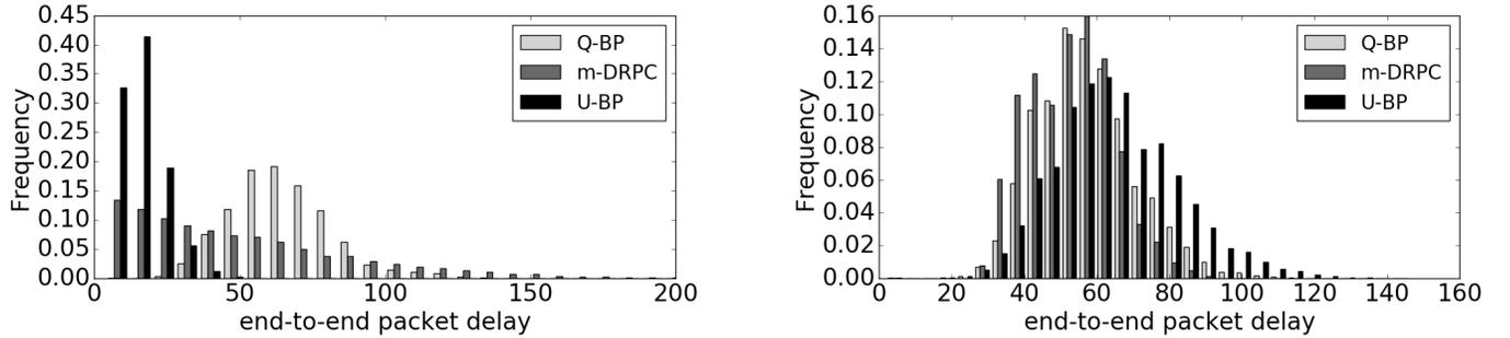
(a) High-priority flows. The average delay in time slots is 64.4 for  $Q$ -BP, 65.7 for  $m$ -DRPC and 15.7 for  $U$ -BP.
