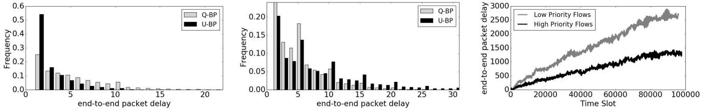
(a) High-priority flows with  $Q$ -BP and  $U$ -BP. The mean delays are 5.354 and 3.004 time slots, respectively. (b) Low-priority flows with  $Q$ -BP and  $U$ -BP. The mean delays are 5.615 and 8.107 time slots, respectively. (c) The  $m$ -DRPC algorithm leads to an unstable network with increasing delays as a function of time.
