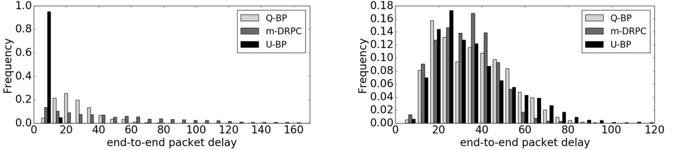
(a) High-priority flows. The average delay in time slots is 27.54 for  $Q$ -BP, 53.4 for  $m$ -DRPC and 7.18 for  $U$ -BP.
