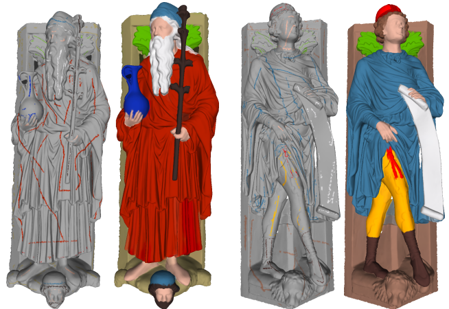
Figure 8: Only a few scribbles are needed to colorize the cloth, despite its folded structure. Note how the fingers are separated from the folded cloth or the hand-held objects.
