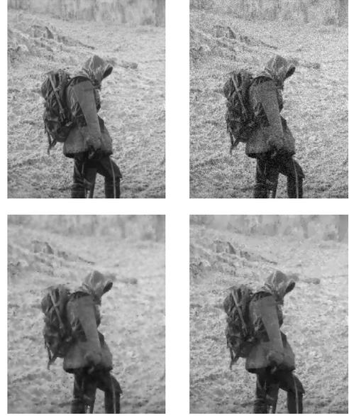
Fig. 7. Comparison between regularized Perona-Malik and our adaptive scheme. Top: original (left), image contaminated by additive white Gaussian noise (right,  $\sigma = 15$ ). Bottom: image denoised using regularized Perona-Malik (P-M) (left) and processing with adaptive  $\lambda$ . Textures and small scale features are kept better in our scheme.
