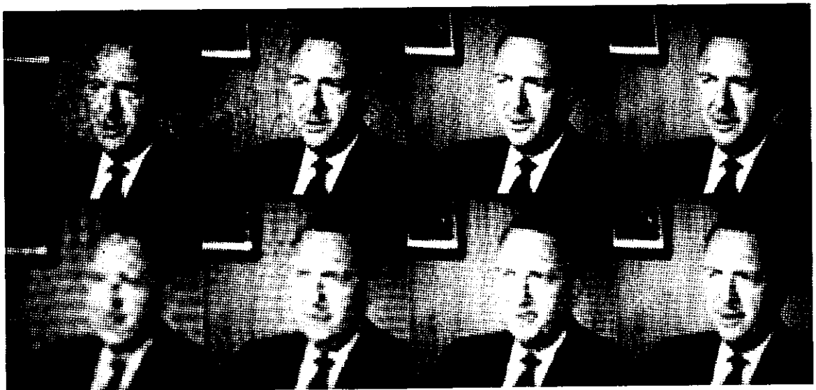
FIG. 1. Gabor decomposition and reconstruction from a partial set of coefficients. Top row: using Zak transform. Bottom row: using biorthogonal dual (gamma) functions. The sequence from left to right corresponds to 600, 1000, 3000, and 9000 coefficients.
