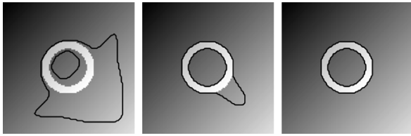
Fig. 11. (Left and middle) Curve's evolution represents the combined influence of both mechanisms. (Right) Application of the combined approach results in an accurate detection.
