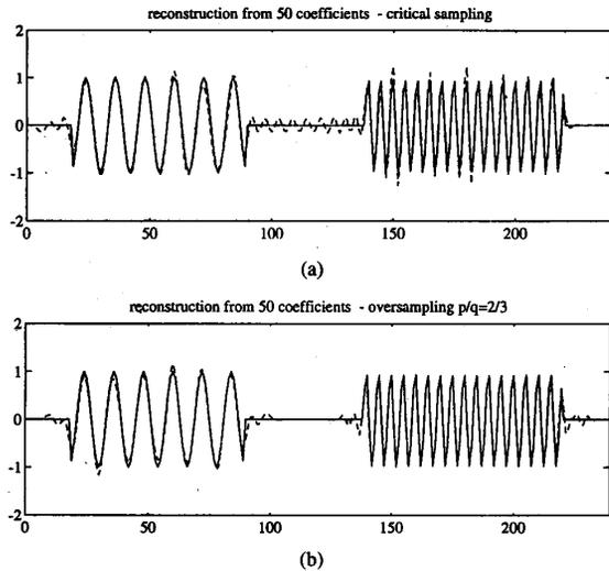
Fig. 2. Signal reconstruction from partial information of the Gabor expansion coefficients. Reconstruction (approximations) of the signal shown in Fig. 1(a) are compared by using the 50 coefficients of the highest magnitude: (a) Reconstruction in the case of critical sampling; (b) reconstruction in the case of oversampling. Note the better reconstruction and separation of the two tones obtained from the same number of coefficients in the case of oversampling.
