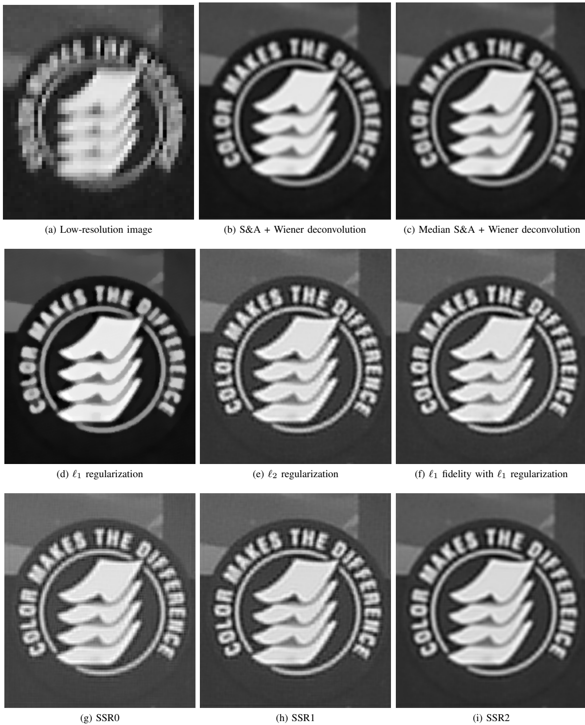
Fig. 9: Resolution enhancement by a factor of \Delta = 4 from a set of 20 images.
