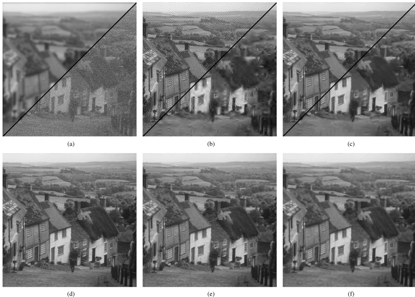
Fig. 4. Deblurring with a blurred/noisy image pair using PLMMSE estimation and RD [7]. (a) Blurred image Y (top left) and noisy image Z (bottom right). (b) LMMSE-deblurred image \hat{X}_Y^L (top left) and MMSE-denoised image \hat{X}_Z^{NL} (bottom-right). (c) BM3D-deblurred image (top left) and BM3D-denoised image (bottom-right). (d) Original image X . (e) PLMMSE estimate \hat{X}^{PL} from Y and Z . (f) RD recovery from Y and Z .
