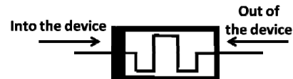
Figure 1. Memristive device symbol. The thick black line on the left side of the device represents the polarity of the device. If the current flows into the device, the resistance of the device decreases. If the current flows out of the device, the resistance increases.
