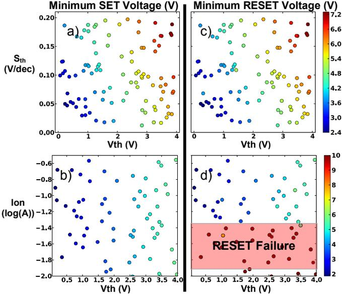
Fig. 5. Simulation results of minimum SET and RESET voltages for 1S1R cells (absolute value shown by the color scale (V)): (a-b)  $V_{MINS}$  and (c-d)  $V_{MINR}$ . For (a)(c),  $I_{th} = 1$  pA,  $I_{on} = 100$  mA, and  $S_{on} = \infty$  V/dec; For (b)(d)  $I_{th} = 1$  pA,  $S_{th} = 0.01$  V/dec, and  $S_{on} = \infty$  V/dec.
