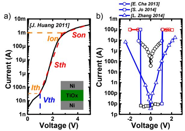
Fig. 4. (a) Five-parameter selector characteristics illustration, where  $V_{th}$  and  $I_{th}$  imply *L*-region selector behavior,  $S_{th}$  captures *T*-region behavior and  $I_{on}$  and  $S_{on}$  indicates *S*-region behavior. (b) Reported selectors can be described using this characterization. The black line is *L*-region, blue line is *T*-region and red line is *S*-region.
