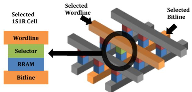
Fig.2. Schematic of a 1S1R crossbar array.
