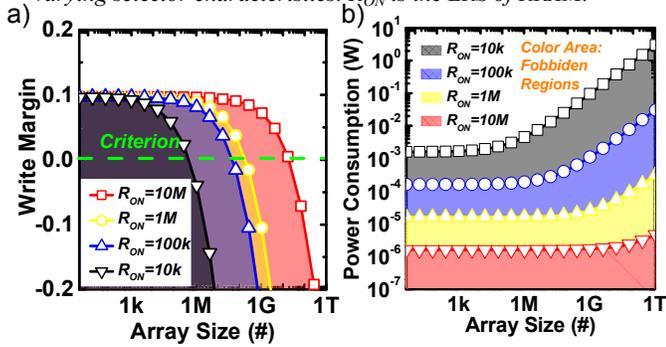
Fig. 8. (a) Envelope of write margin attainable by using optimal selector characteristics. For each RRAM with different LRS, the corresponding color space of write margin can be attained by varying selector characteristics. (b) Envelope of energy consumption not attainable by using optimal selector characteristics. For each RRAM with different LRS, the corresponding color space of energy consumption cannot be attained by varying selector characteristics.
