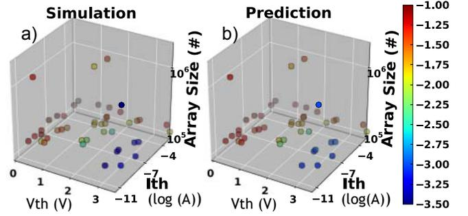
Fig. 6. Simulation (a) and prediction (b) results of 1S1R array ( $512 \times 512$  and  $1024 \times 1024$ ) RESET power consumption for test data. The color scale represents the logarithm of power consumption ( $\log(W)$ ). The unit of  $V_{th}$  and  $I_{th}$  is V and  $\log_{10}(A)$  respectively.
