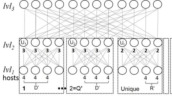
**Figure 6: An example of host placement with  $N = 32$  hosts on a 3-level fat-tree using the *Approximated* method. Using a notation similar to the 2-level fat-tree, this allocation is of the form:  $Q' = 2$ ,  $D' = 3$  and  $R' = 2$ .**
