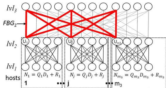
**Figure 5: A 3-level fat-tree showing the host allocation on each 2-level sub-tree matching Theorem 1. One of the  $lvl_2 - lvl_3$  Full Bipartite Graphs ( $FBG_2$ ) is highlighted. We denote as  $U_j$  the maximal number of flows injected into this  $FBG_2$  from the  $j^{th}$  2-level sub-tree.**
