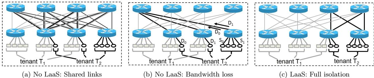
**Figure 1: Two tenants hosted on a cloud. (a) Their traffic interferes on many shared links. (b) There are no shared links, but the second tenant cannot service an admissible traffic from  $S_0$  and  $S_1$  to  $D_0$  and  $D_1$ . (c) Under LaaS conditions of tenant placement and link allocation, the network can service any admissible tenant traffic demands.**
