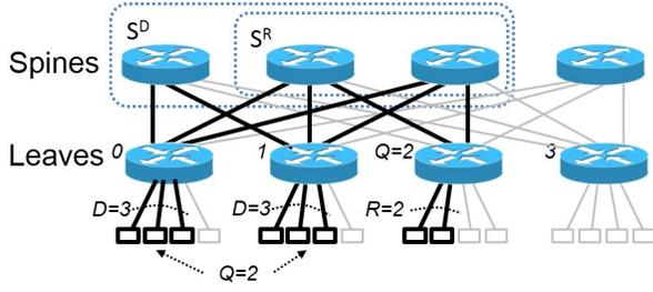
**Figure 3: A tenant of  $N = 8 = Q \cdot D + R$  hosts. To implement LaaS, there must be  $Q$  leaves of  $D$  hosts and optionally one leaf of  $R < D$  hosts.**
