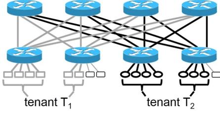
**Figure 2: Two tenants of sizes 6 and 7 hosts placed by the *Simple* heuristic, where each tenant fills a number of complete sub-trees.**
