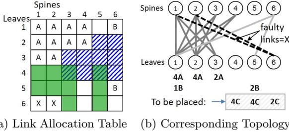
**Figure 7: Example of allocation with 2 potential placements.** (a) Table of leaf up-links holding the link assignments of tenants A and B, as well as 2 faulty links X. (b) Corresponding topology. The new tenant C of 10 hosts, arranged as  $Q \cdot D + R = 2 \cdot 4 + 2$ , can be assigned one of two allocations. In (a), the first link allocation is shown in solid, and the second with slanted lines.
