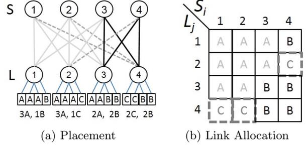
**Figure 4: Illustration that a simple host placement is not sufficient, and a joint host placement and link allocation is necessary for LaaS. (a) All tenants satisfy the host placement necessary conditions, e.g. the placement of C is  $3 = Q \cdot D + R = 2 \cdot 1 + 1$ . A and B support any admissible traffic matrix by the sufficient link allocation conditions. (b) However, the link allocation for C is impossible. There is no way to find a common set of spines with free ports.**
