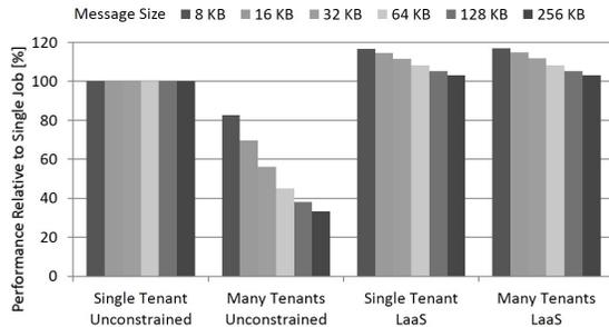
Figure 11: Simulated relative performance for tenants running Stencil scientific-computing applications on a cloud of 1,728 hosts, either alone or as 32 concurrent tenants. While tenant performance degrades when placed unconstrained (without link isolation), the performance of single and multiple tenants with LaaS appears identical, fulfilling the promise of LaaS.
