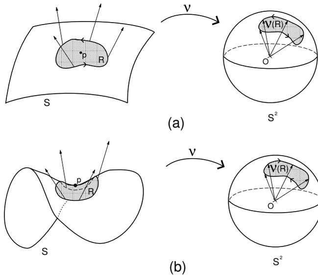
Figure 2: Gauss Curvature Definition: (a)  $K(p) > 0$  and (b)  $K(p) < 0$
