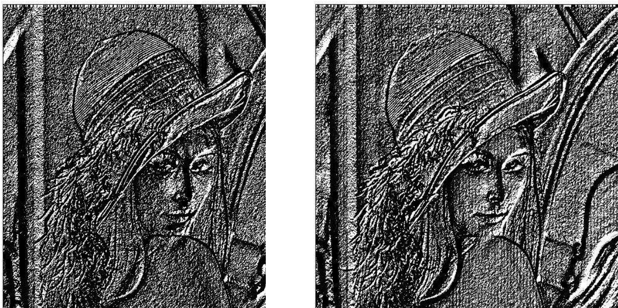
Figure 3: Curvatures Maps: Left - Green channel, Right - Red channel. The images above show the Gaussian curvature in two different channels yet they look almost the same.
