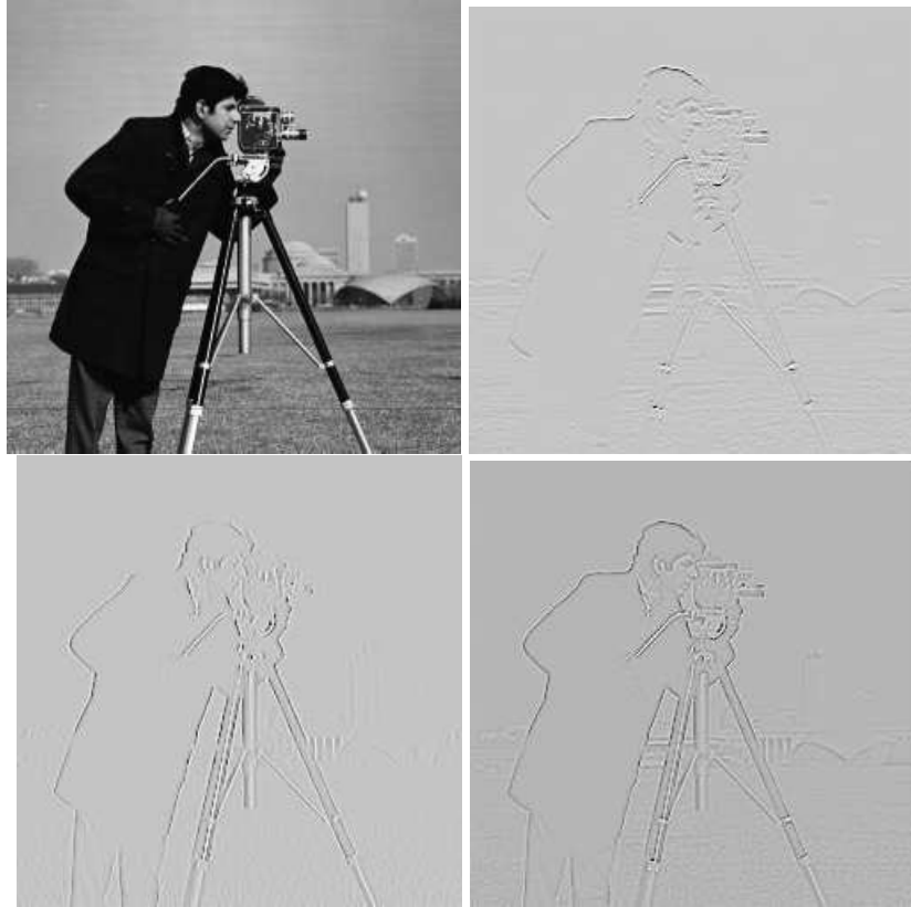
Fig. 4. Computing the Ricci curvature for a pixel: The “Camera Man” test image (top, left), Ricci curvature computed in horizontal (top, right) and vertical (bottom, left) directions, and the Ricci (averaged) curvature (bottom, right).
