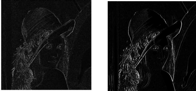
Fig. 5. Gauss (left) and Combinatorial Ricci (right) comparison. Note the edge detecting capability of the Combinatorial Ricci curvature.
