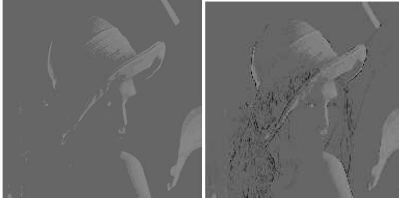
Fig. 6. Comparison of Different Laplacians: The Combinatorial (Forman) Laplacian \square_1(e_0) (left), and the Bochner (rough) Laplacian B_1(e_0) (right). Note that the combinatorial Laplacians are good detectors of “sharp” edges.
