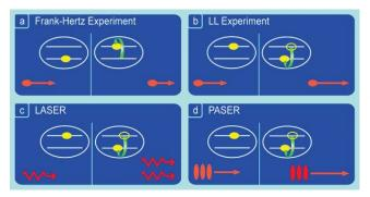
The electrons stimulate the atoms into giving up their surplus energy through collisions. The electrons' energy is amplified in a coherent way. Although millions of collisions are involved for each electron, no heat is generated. The transferred energy goes into an enhanced electron motion. One could say that here was a laser
