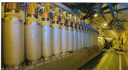
Now that the first of the large feedboxes is in, sector 7-8 is preparing to cool down.
