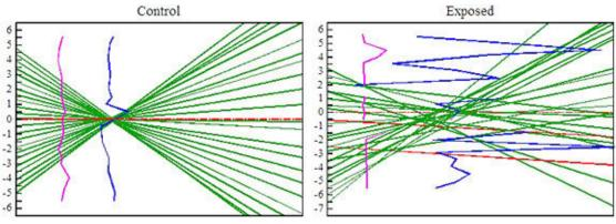
Good quality lens as demonstrated by the optical scanner. All rays passing Through the lens have similar focal length. The thick dashed line connects the points of the back vertex Distance for each ray passing through the lens. The thick solid line shows the relative intensity of each beam.
