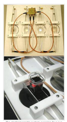
The electromagnetic system exposing four eye lenses to electromagnetic radiation Each vessel containing a lens, inserted between the two plates of the transmission line. The entire system is placed in an incubator maintaining constant temperature for the duration of exposure.
