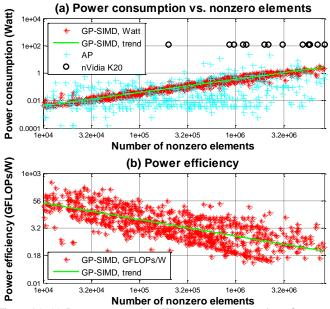
Figure 15. (a) Power consumption (Watt) vs. average number of nonzero elements per row. (b) Power efficiency (GFLOPs/W) vs. average number of nonzero elements per row
