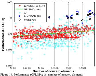
The performance the GP-SIMD SpMM, AP, and two commercial processors (Intel XEON-PHI and K20 [10]) as functions of the number of nonzero elements is presented in Figure 14, and the simulated power consumption of the GP-SIMD SpMM, and AP (as well as reported power of NVidia K20 [34]) is presented in Figure 15(a).
