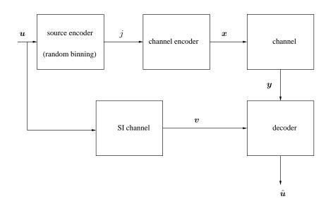
Figure 1: Slepian–Wolf source coding, followed by channel coding. The source u is source–channel encoded, whereas the correlated SI v (described as being generated by a DMC fed by u) is available at the decoder.
