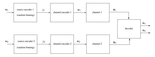
Figure 2: Separate source-channel encodings and joint decoding of two correlated sources.
