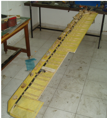
Figure 38: Wing Bending NDT
