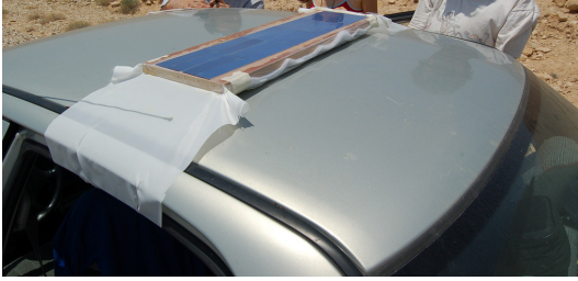
Figure 40: Solar Array Wind Cooling Test.
