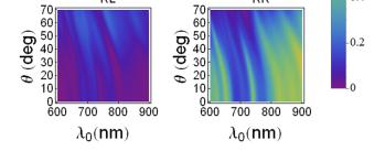
**Figure 6** Measured spectrums of the four circular transmittances of the dual-band circular-polarization filter for  $\theta \in [0^{\circ}, 70^{\circ}]$ . [Color figure can be viewed in the online issue, which is available at wileyonlinelibrary.com.]
