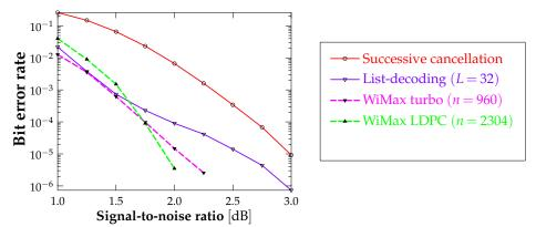
Simulation results for a polar code of length n = 2048 and rate R = 0.5, optimized for a BPSK-AWGN channel with  $E_b/N_0 = 2.0$  dB.
