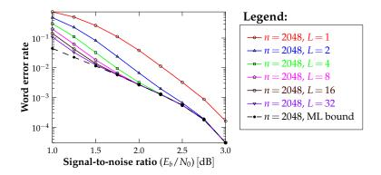
List-decoding performance quickly approaches that of maximum-likelihood decoding as a function of list-size.
