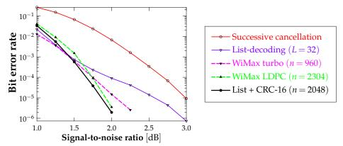
Polar codes (+CRC) under list decoding are competitive with the best LDPC codes at lengths as short as n = 2048.
