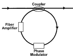
Fig. 3. Schematic of an experimental realization of the fiber kicked system in a loop configuration as repeated modulations and kicks are applied as a pulse circulates in the loop.
