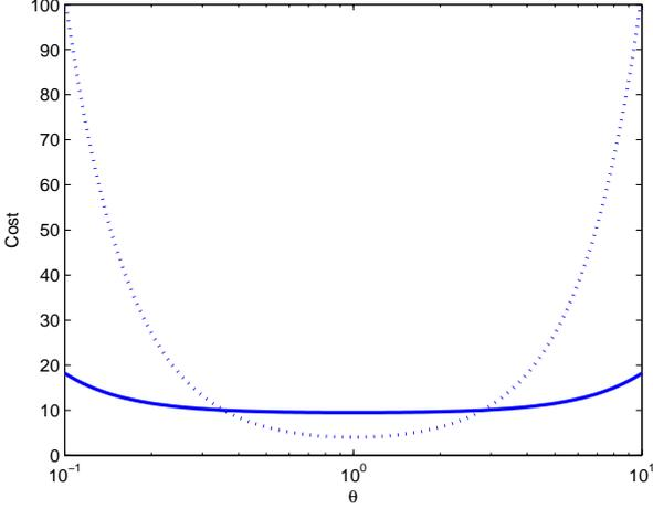
Fig. 1.  $[\theta^2 \overline{M}(\theta, \phi_u)]^{-1}$  as a function of  $\theta$  for nominal input (dotted) and ‘1/f’ noise (solid).
