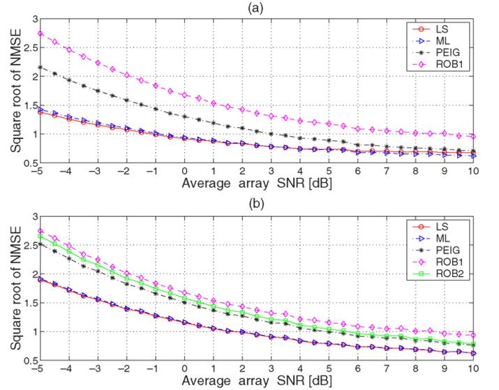
Fig. 2. Square root of the normalized MSE as a function of average array SNR for nondiagonal  $\mathbf{C}$ . (a) Assuming known  $\mathbf{m}$  and  $\mathbf{C}$  and using an estimate for  $\mathbf{R}$ . (b) Assuming known  $\mathbf{m}$  and using estimates for  $\mathbf{R}$  and  $\mathbf{C}$ .
