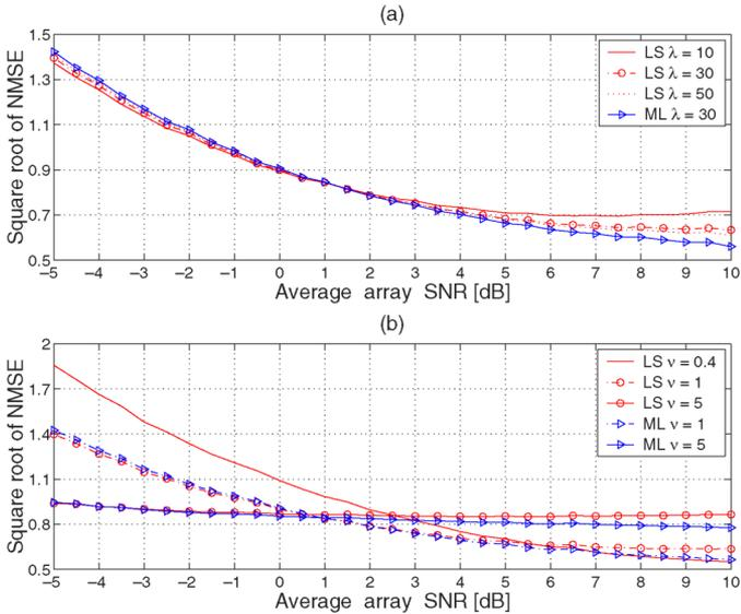
Fig. 3. Square root of the normalized MSE as a function of average array SNR for diagonal  $\mathbf{C}$ . (a) Assuming known  $\mathbf{m}$  and  $\mathbf{C}$  and  $\mathbf{R}$  estimated with three different values for  $\lambda$ . (b) Assuming known  $\mathbf{m}$ ,  $\mathbf{R}$  estimated with  $\lambda = 30$ , and  $\mathbf{C}$  estimated with three different values for  $\nu$ .
