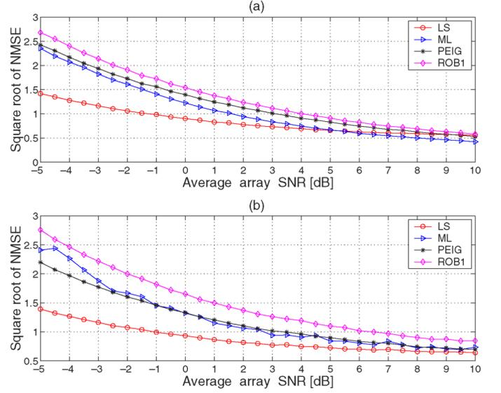
Fig. 1. Square root of the normalized MSE as a function of average array SNR assuming known values of  $\mathbf{m}$ ,  $\mathbf{C}$ , and  $\mathbf{R}$ . (a) Diagonal  $\mathbf{C}$ . (b) Nondiagonal  $\mathbf{C}$ .
