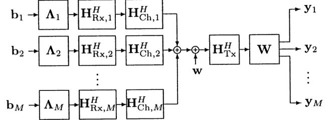
Fig. 3. Block diagram of an uplink (multiple access) system. The matrices  $\Lambda_m$  for  $m = 1, \dots, M$  are diagonal matrices with the  $\lambda_i$ 's associated with  $\mathbf{b}_m$ . The vector  $\mathbf{w}$  is the virtual uplink noise vector.
