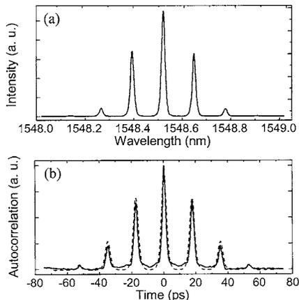
Fig. 2. (a) Measured spectrum of the periodic phase modulation function induced by EO modulation of CW light with a sinusoidal waveform of frequency 16 GHz and a modulation index of 1.24 rad (a.u. is arbitrary units). (b) Measured autocorrelation of the generated optical pulse sequence (solid curve) and numerically calculated autocorrelation of the measured comb spectrum in (a) (dashed curve).
