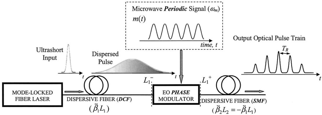
Fig. 1. Schematic of the proposed fiber-based programmable optical pulse burst generator.
