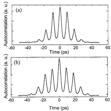
Fig. 4. Measured autocorrelation of the generated optical pulse sequence with a sinusoidal modulation waveform of frequency 8 GHz and a modulation index of (a) 1.24 rad, (b) 1.62 rad.
