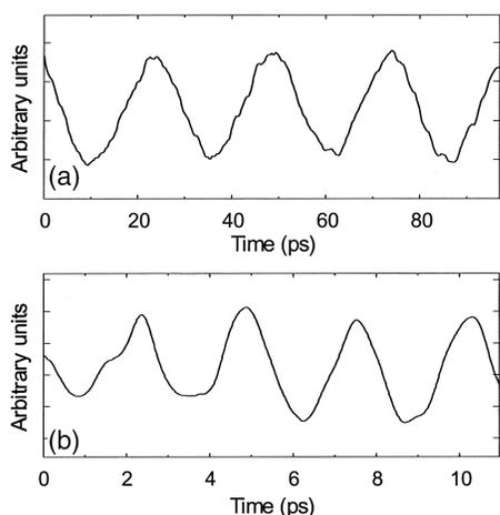
Fig. 4. Autocorrelation traces that correspond to the optical signals measured (a) before and (b) after the second dispersive stage when the TI system is configured for achieving  $M_t = 0.113$ , with  $f_1 = 40$  GHz.
