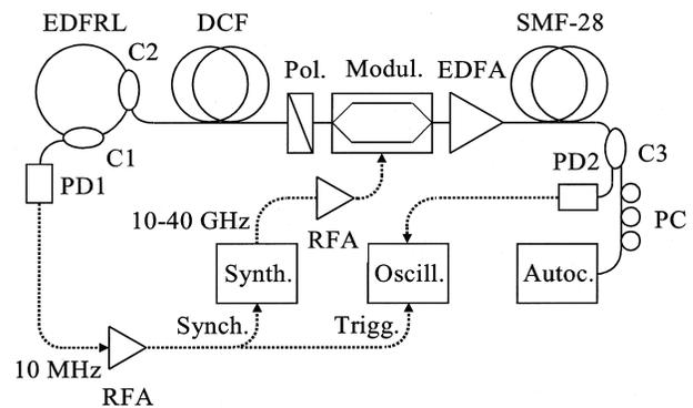
Fig. 2. Experimental setup: EDFA, erbium-doped fiber amplifier; C3, fiber coupler; PC, polarization controller; other notation defined in text.
