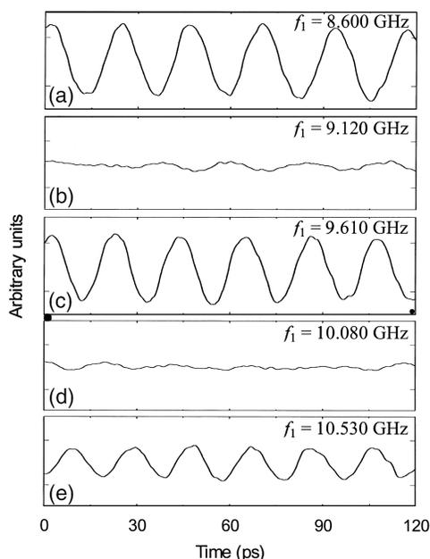
Fig. 3. Measured microwave signals at the output of the TI system (image magnification factor,  $M_t = 0.2$ ) for several input modulation frequencies ( $f_1$  near 10 GHz).
