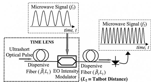
Fig. 1. Schematic of the proposed microwave frequency-shifting technique based on a general temporal self-imaging (Talbot) effect.
