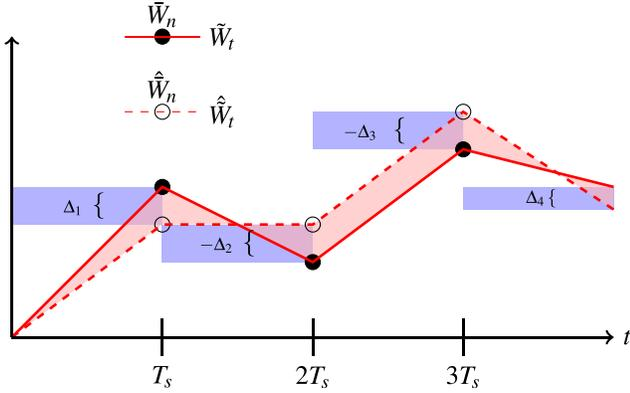
Fig. 10. The error in estimating  $\tilde{W}_{[.]}$  and  $\tilde{W}_{(.)}$  corresponds to the blue and red areas, respectively. Negatively correlated  $\Delta_n$  and  $\Delta_{n+1}$  are preferred for minimizing the distortion with respect to  $\tilde{W}_{(.)}$ , while the distortion with respect to  $\tilde{W}_{[.]}$  is indifferent to this correlation.
