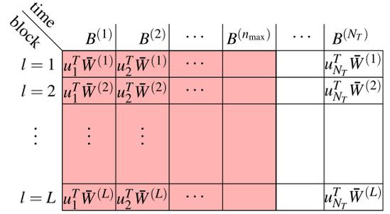
Fig. 8. Description of encoding  $\bar{W}^{LN_T}$  using the encoder  $\bar{f}_{NL}$ : divide the vector  $\bar{W}^{LN}$  into the length  $N$  blocks  $\bar{W}^{(1)}, \dots, \bar{W}^{(L)}$  defined in (43). For  $n = 1, \dots, N$ , form the vector  $B^{(n)}$  consisting of the  $n$ th coefficient in the KL transform of each of the  $L$  blocks. Each such vector is encoded using a random Gaussian codebook of rate  $L\bar{R}_n$  bits;  $\bar{R}_n = 0$  for  $N > n_{\max}$ .
