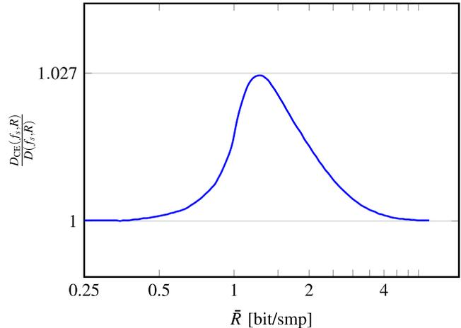
Fig. 9. The ratio  $D_{\text{CE}}(f_s, R)/D(f_s, R)$  versus  $\bar{R} = R/f_s$  describing the performance loss in using CE compared to the optimal source coding scheme.
