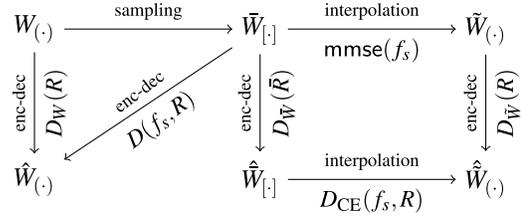
Fig. 4. Relations among the processes  $W_{(\cdot)}$ ,  $\bar{W}_{[\cdot]}$ ,  $\tilde{W}_{(\cdot)}$  and their associated distortion functions. Each reconstruction operation is associated with a distortion quantity. In this paper we show that  $D_{\tilde{W}}(R) \leq D_{\tilde{W}}(R/f_s) \leq D(W_{(\cdot)} | \bar{W}_{[\cdot]}) \leq D(f_s, R) \leq D_{CE}(f_s, R) \leq \text{mmse}(f_s) + D_{\tilde{W}}(R/f_s)$ , where  $D(f_s, R) = \text{mmse}(f_s) + D_{\tilde{W}}(R)$ .
