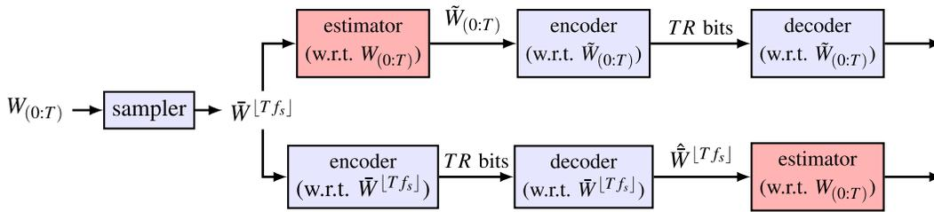
Fig. 2. Two source coding approaches. Upper Path: Estimate-and-Compress (EC). Lower Path: Compress-and-estimate (CE). EC achieves the minimal distortion in the combined sampling and source coding problem of Fig. 1. CE does not require parameters of the continuous-time model at the encoder.
