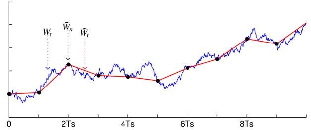
Fig. 3. Sample paths of a Wiener process  $W_{(\cdot)}$ , its discrete-time samples  $\bar{W}_{[1]}$ , and its conditional expectation given these samples  $\tilde{W}_{(\cdot)}$ .
