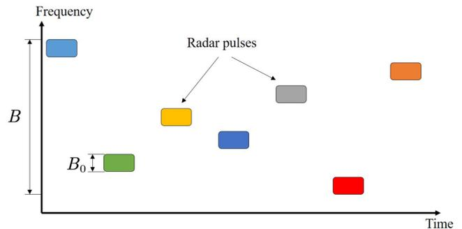
Fig. 1. An example of a FAR waveform. The boxes indicate the frequency band transmitted in the given time window.
