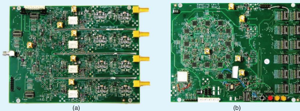
**[FIG12]** A hardware realization of the MWC consisting of two circuit boards. Part (a) implements  $m = 4$  sampling channels, whereas (b) provides four sign-alternating periodic waveforms of length  $M = 108$ , derived from a single shift-register. Adapted from [47] (figure courtesy of IET).
