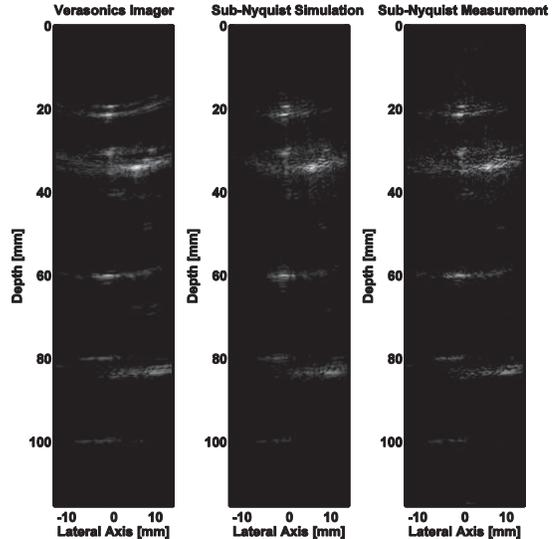
Figure 6: Comparison between a conventional full-rate beamformed image (a) and the simulated sub-Nyquist AFE performance given measured full-rate data (b). Image (c) is the measured sub-Nyquist AFE reconstruction from the same transmit event. Images (b) and (c) were generated using a factor of 43 less data than image (a).
