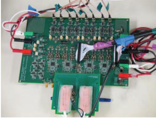
Figure 2: PCB implementation of the sub-Nyquist AFE. The sub-Nyquist AFE measures 7.5x10.8 inches in size, and implements 32 receiving channels.
