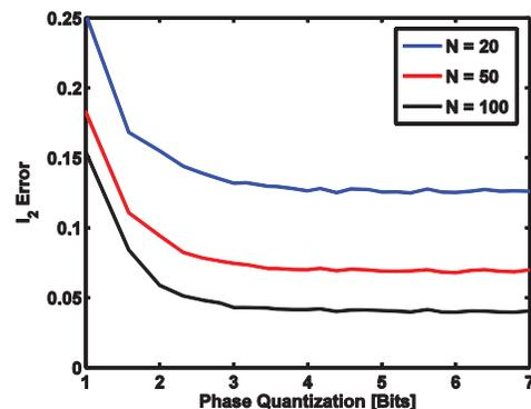
Figure 4: Simulated characterization of phase quantization on reconstruction accuracy. While overall beamforming accuracy is dictated by the number of samples taken for frequency-domain beamforming, error introduced by phase quantization is limited after 4 bits.
