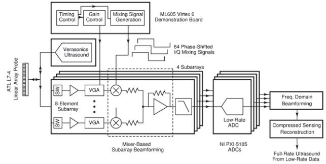
Figure 3: System architecture for sub-Nyquist sampling AFE. Transmit operation is controlled by the Verasonics machine. Reflected signals are received simultaneously by the Verasonics and sub-Nyquist AFEs.
