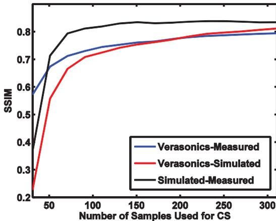
Figure 7: Characterization of sample count on the resulting reconstructed image SSIM when compared against a full-rate signal. A smooth tradeoff exists between sample count and image accuracy, and a high level of agreement is found between the reconstructions from simulation and measured data.
