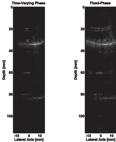
Figure 5: Images reconstructed from low-rate samples measured with the sub-Nyquist sampling AFE. Figure (a) implements subarray beamforming using time-varying phase in the mixing signals as in [9], (b) uses fixed-phase mixing sequences instead.
