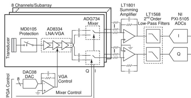
Figure 1: Subarray architecture for sub-Nyquist sampling AFE. 8 channels are beamformed using mixer-based beamforming and summed prior to digitization.
