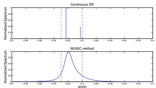
Fig. 4: Resolution capability using CSR and MUSIC algorithm, with  $\text{SNR} = -5\text{dB}$ ,  $T = 500$ .
