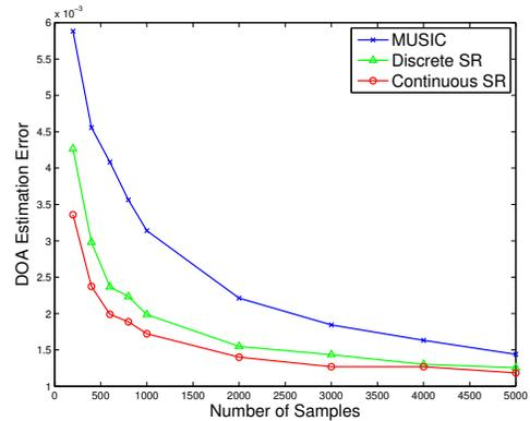
Fig. 3: DOA estimation error for CSR, MUSIC, and DSR, with  $\text{SNR} = -10\text{dB}$ .
