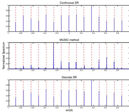
Fig. 1: Normalized spectra for CSR, MUSIC, and DSR, with  $T = 500$  and  $\text{SNR} = -10\text{dB}$ .
