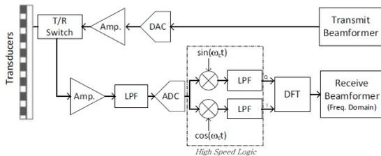
Fig. 5: Transmit and receive paths of medical ultrasound system with beamforming in the frequency domain.
