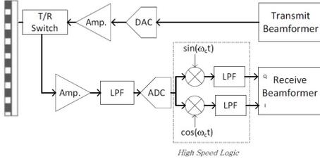
Fig. 2: Transmit and receive front-end of state-of-the-art medical ultrasound system.
