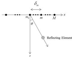
Fig. 1:  $M$  transceivers aligned along the  $x$  axis, with an acoustic pulse transmitted at direction  $\theta$ .
