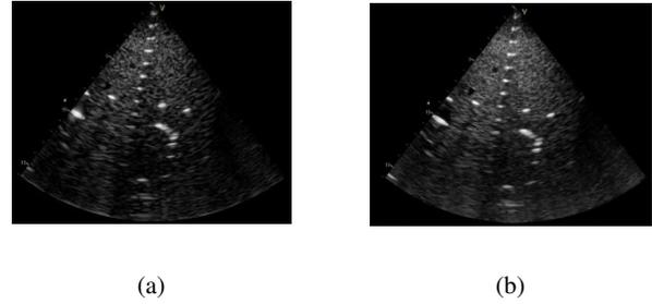
Fig. 6: Phantom images obtained by (a) Beamforming in frequency at a low rate (b) Beamforming in time at a standard rate
