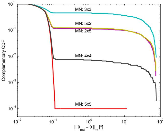
Fig. 3. CCDFs for the truncated BB algorithm parametrized by the number of transmit/receive elements.
