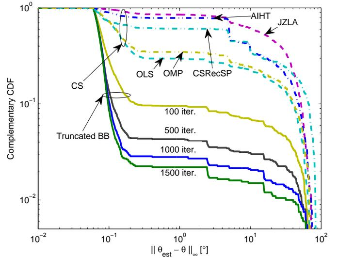
Fig. 1. CCDFs of the truncated BB algorithm with different termination criteria.
