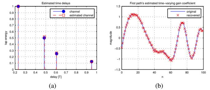
**Fig. 3.** Channel estimation with  $p = 5$  and SNR=20dB. (a) delays recovery. (b) Estimated first path time-varying gain coefficient.
