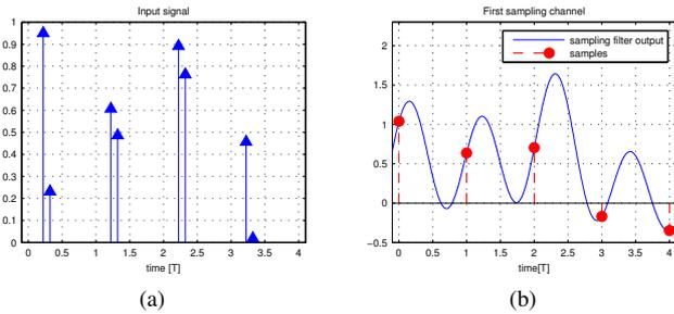
**Fig. 2.** Stream of Diracs. (a)  $K = 2$  Diracs per period. (b) First sampling channel output.
