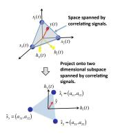
Fig. 3: The projection performed by RD-MUD. The figure illustrate the case N = 3, M = 2, and the received signal is due to two active users.
