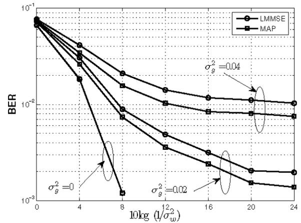
Fig. 3. Bit error rate of a MIMO system with  $N = 40$ ,  $K = 4$  for various values of  $\sigma_g^2$ .
