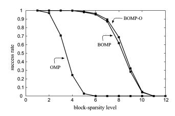
Fig. 3. Performance of OMP, BOMP, and BOMP-O for a dictionary with L = 80, N = 160, and d = 8.
