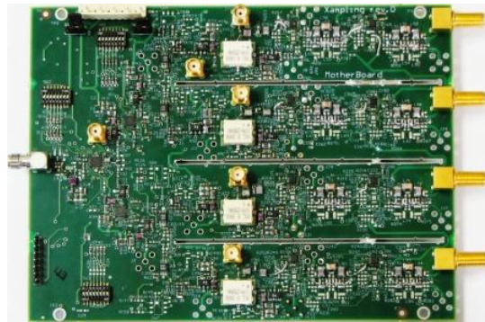
Fig. 11. The analog board realizing four sampling channels. It consists of three stages: splitting the analog input, mixing with four input periodic waveforms (connectors on the rear), and lowpass filtering.
