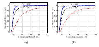
Fig. 8. Percentage of correct support recovery, when drawing the sign patterns randomly only for the first r channels. Results are presented for (a) SNR=25 dB and (b) SNR=10 dB.
