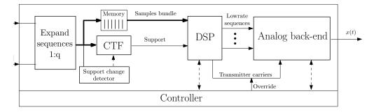
Fig. 6. High-level architecture for efficient multiband reconstruction.
