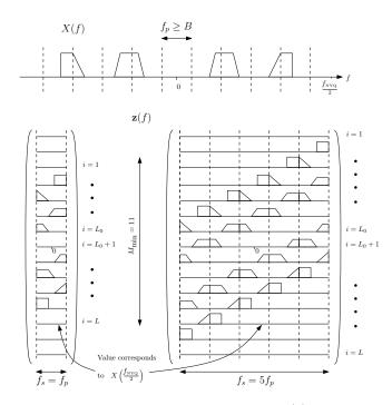
Fig. 4. The relation between the Fourier transform X(f) and the vector set  $\mathbf{z}(f)$  of (13). In the left pane,  $f_s = f_p$  so that the length of  $\mathbf{z}(f)$  is L = 11. The right pane demonstrates  $f_s = 5f_p$  which gives L = 15. Entries in locations  $i \leq L_0$  ( $i > L_0 + 1$ ) contain shifted and windowed copies of X(f) to the right (left) of the frequency axis. No shift occurs for the middle entry,  $i = L_0 + 1$ .
