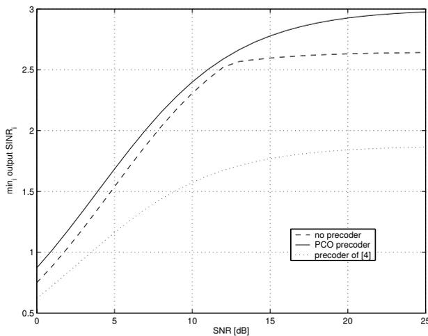
Fig. 3. Worst output SINR in a system with  $K = 4$  and  $N = 3$ .
