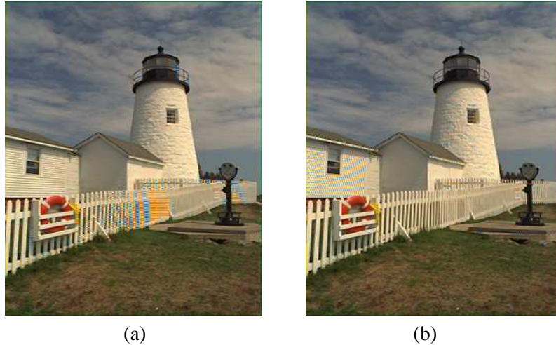
Fig. 13. The output of the red and blue estimation stage (a) horizontal interpolation (b) vertical interpolation.
