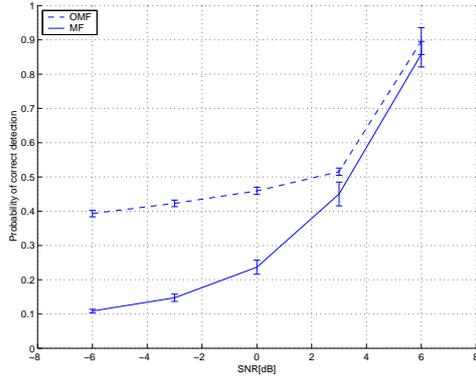
**Fig. 1.** Mean  $P_D$  using the OMF and MF detectors in Beta-distributed noise, as a function of SNR. The vertical lines indicate the standard deviation of the corresponding  $P_D$ .
