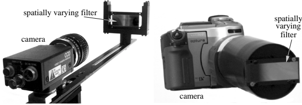
Figure 2. Two generalized mosaicing systems. [Left] A system composed of a Sony black/white video camera and an extended arm which holds the filter. [Right] A system that includes a Canon Optura digital camera and a cylindrical attachment that holds the filter. In both cases, the camera moves with the attached filter as a rigid system.
