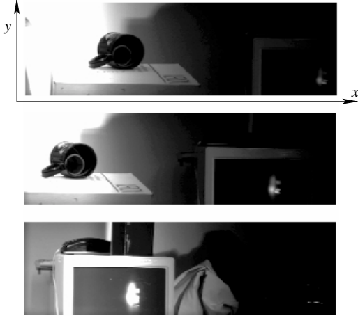
Figure 3. Images taken with the linear variable density filter. Scene features become brighter as they move leftwards in the frame. Bright scene points gradually reach saturation. Dim scene points, which are not visible in the right hand side of the frames, become visible when they appear on the left.
