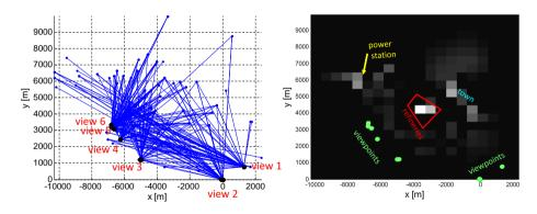
**Fig. 9.** [Left] Experimental setup of the outdoor experiment. Black dots indicate view-points. Any blue line represents a ray between a viewpoint and an object point. Figure axes are aligned to the compass cardinal directions in our region. [Right] The estimated TS parameter  $C_n^2$  shown in a 2D map. Bright areas represent high values while dark areas represent low values. Regional places of interest are overlayed on the map. Notice the hottest spot is at the oil refineries.
