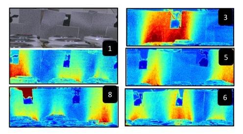
**Fig. 3.** Sample variance images from an experiment corresponding to Fig. 6. A textured pattern which is placed behind the stove is shown aligned with its variance image, from one view. Sample variance images of pixel displacements, in various views, with corresponding camera indices. Red expresses high variance while blue represents low variance. High variance regions appear only behind hot stoves.
