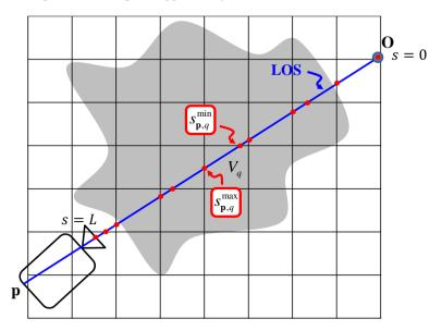
**Fig. 4.** The volume is discretized into voxels. The LOS intersects voxel  $V_q$  at points  $s_{\mathbf{p},q}^{\min}$  and  $s_{\mathbf{p},q}^{\max}$ . The voxel intersection points  $\Psi_{\mathbf{p},q} \equiv \mathrm{LOS}_{\mathbf{p}} \cap V_q$  are used as weights in the LOS integration (9).
