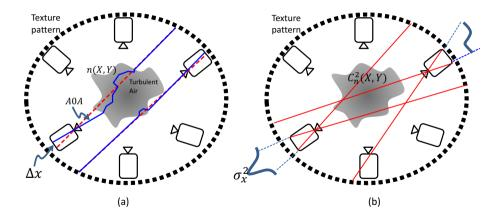
Fig. 1. Multiple cameras are placed around a chunk of turbulent air. (a) An object point of a textured pattern projects to a camera pixel through air having a spatially varying refractive index. (b) Temporal variance of pixel displacement of a textured object is associated to a pixel. This yields data for linear tomography of the statistical field  $C_n^2$ .
