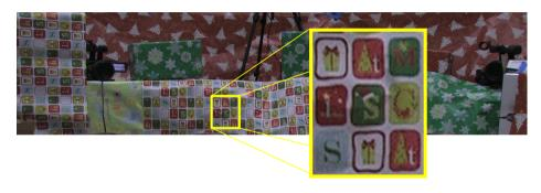
Fig. 2. An example of an image frame as seen through turbulent air. Notice the distorted edges in the magnified region.
