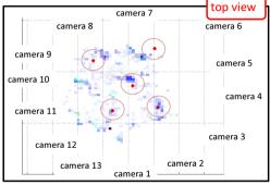
**Fig. 6.** [Left] Laboratory experimental setup. Multiple cameras encircle hot electric cooking stoves which create turbulence. Sample variance images from different viewpoints are shown in Fig. 3. [Right] Top view of an estimated  $C_n^2$ . Red dots indicate the true locations of hot operating stoves. Camera locations are also shown.
