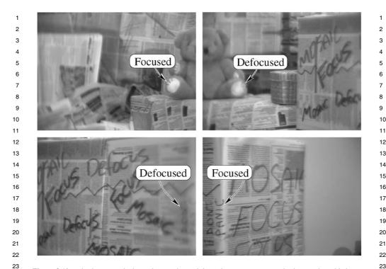
Figure 8.10 The frame in which an object is focused depends on its position in the frame. The teddy bear is focused only when it appears on the right-hand side of the frame's FOV. The words 'don't panic' are focused only when they appear in the left-hand side of the frame's FOV.
