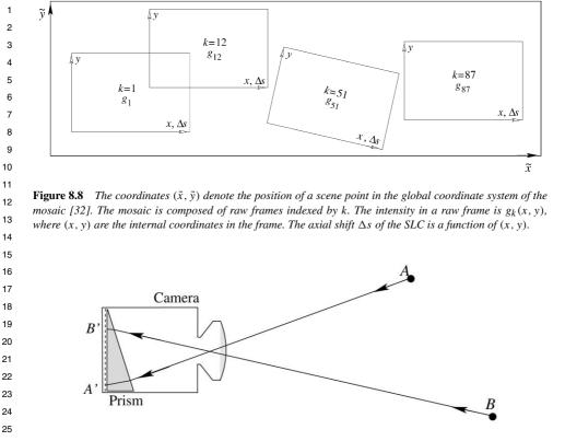
Figure 8.9 The focus settings can change across the frame's FOV by placing a transparent object with variable thickness on the detector. Here, a wedge-prism is placed on the detector array, such that both objects A and B are focused even-though they are at different distances from the camera.
