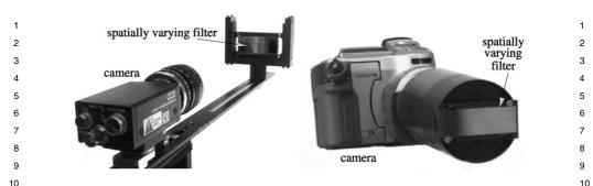
Figure 8.13 Two generalised mosaicing systems [31–33]. (Left) A system composed of a Sony black/white video camera and an extended arm which holds the filter. (Right) A system that includes a Canon Optura digital video camera and a cylindrical attachment that holds the filter. In both cases, the camera moves with the attached filter as a rigid system.
