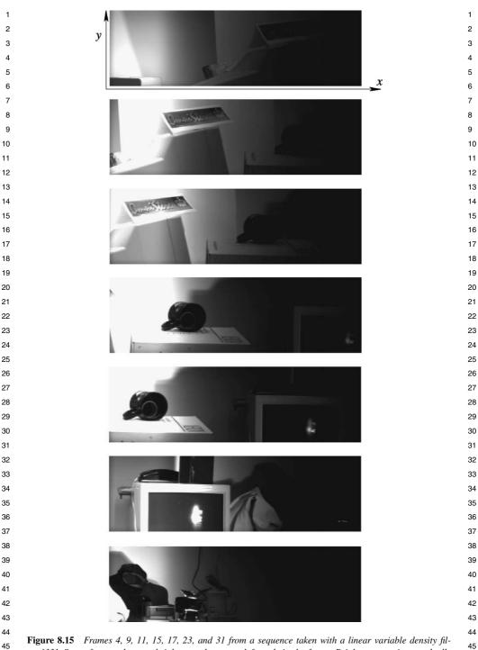
Figure 8.15 Frames 4, 9, 11, 15, 17, 23, and 31 from a sequence taken with a linear variable density filter [33]. Scene features become brighter as they move leftwards in the frame. Bright scene points gradually reach saturation. Dim scene points, which are not visible in the right-hand side of the frames, become visible when they appear on the left.
