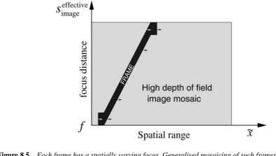
**Figure 8.5** Each frame has a spatially varying focus. Generalised mosaicing of such frames extends both the FOV and the DOF.
